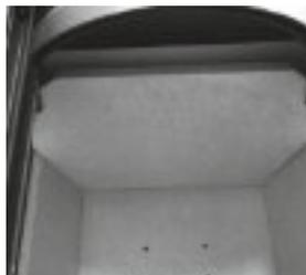
Baffle in position resting on supports.
